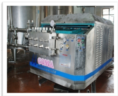
Homogeniser High Pressure Pump 10,000 LPH (GOMA)
